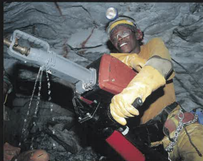
An electric rockdrill – potentially more environmentally – and worker-friendly than traditional pneumatic drills – being tested at AngloGold's Kopanang mine. Photo courtesy AngloGold
