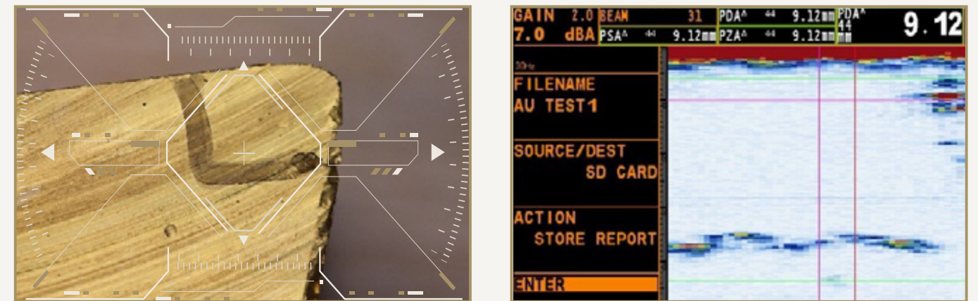
Gold bar with microscopic air pockets which resulted in a failed ultrasound report
