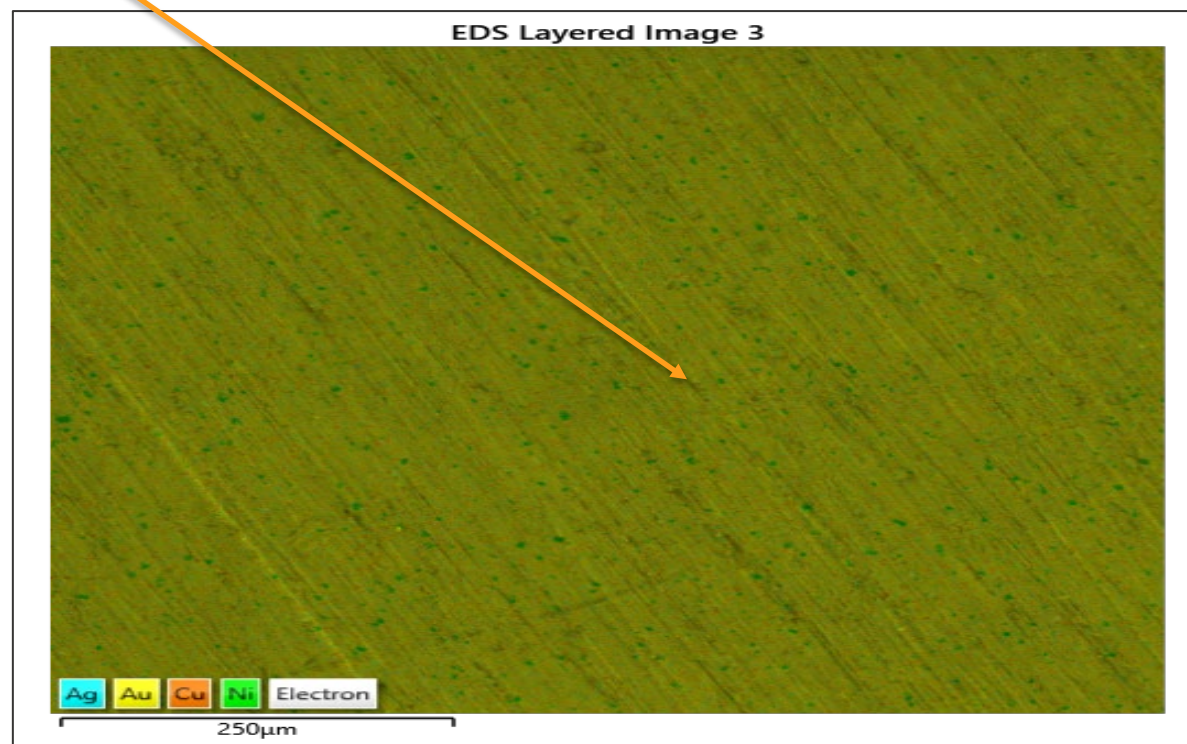
EDX CHEMICAL MAP OF THE BULLION DISC AT A MAGNIFICATION OF 200X
