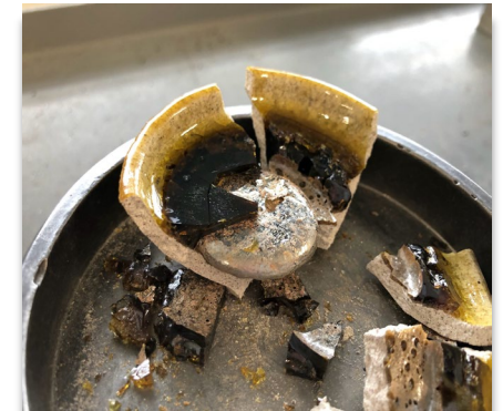
Breaking the scorifier: Extracting the Pb button
