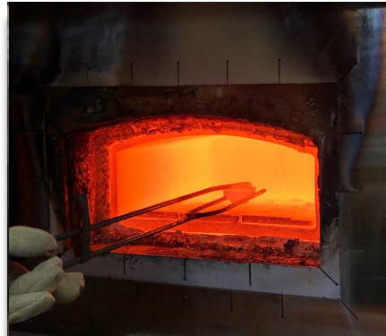
Oxidizing fusion at 1100°C
